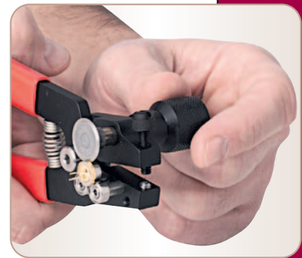
Simple manual can opener removes the cap from most transistor-style laser diode packages.
