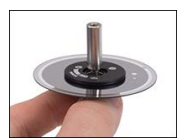
Click to Enlarge Figure 3: Hold Vertically and Secure the Pinhole Wheel
