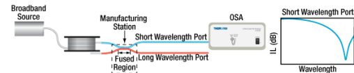
Click to Enlarge In the diagram, the fibers are color-coded; blue for the short wavelength port and red for the long wavelength port.
