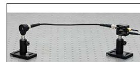
Click to Enlarge The PBM42 Bias Module Used to Apply an External Reverse Bias Voltage to the SM1PD2A Photodiode
