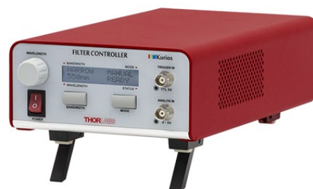
Click to Enlarge The front panel of the KURIOS-WB1/M controller while it is set to manual mode.
