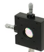
Click to Enlarge Ø1" Optic Mounted in a ST1XY-S XY Translator
