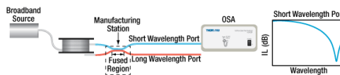
In the diagram, the fibers are color-coded: blue for the short wavelength port and red for the long wavelength port.
