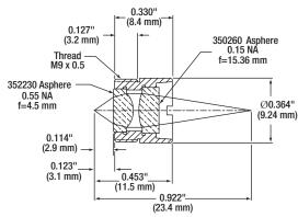
Laser Side: 0.55 NA f = 4.5 mm Fiber Side: 0.16 NA f = 15.36 mm
