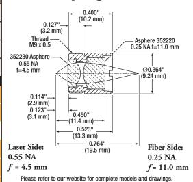
and effective solution for the routine task of coupling a laser diode to a multimode fiber. The laser side of the aspheric lens has a numerical aperture of 0.55 to collimate the highly divergent beam emitted from the laser diode. The multimode fiber side has a numerical aperture of 0.25 to focus the light down. The lens pair is available with an antireflection coating for either 650 to 1050 nm or 1050 to 1620 nm.
