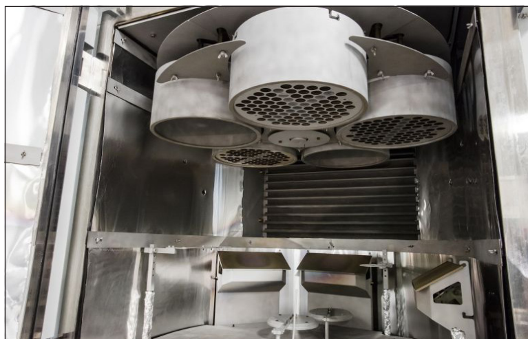
Metallic Mirror Blanks Mounted for Coating in One of Our E-Beam Evaporation Chambers
