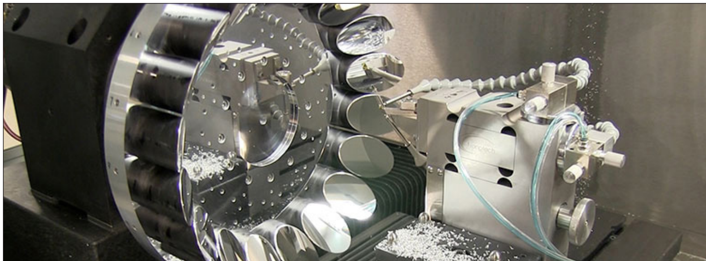
Our Single-Point Diamond Turning Capabilities Allow Us to Produce Custom Off-Axis Parabolic and Aspheric Mirrors
