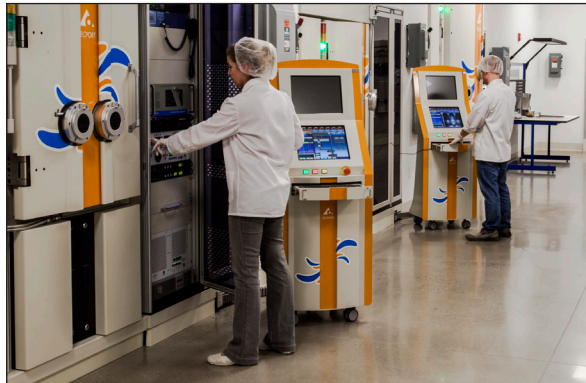
A range of coating techniques to deposit metallic and dielectric coatings are performed by our coating technicians with in-process spectral characterization.
