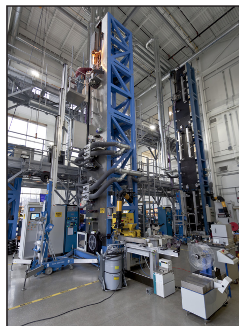
Fiber Being Drawn in Our Fiber Tower
