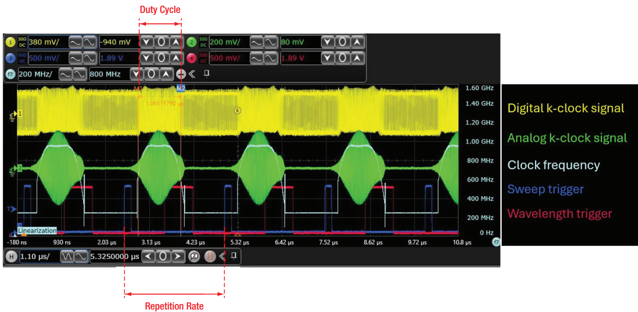
Figure 3: Oscilloscope image of the output signals from an SLZ Series MEMS-VCSEL laser source. These are typical signals for an SLZ1002 with a sweep rate of 1 MHz. The repetition rate and the duty cycle are also shown.
